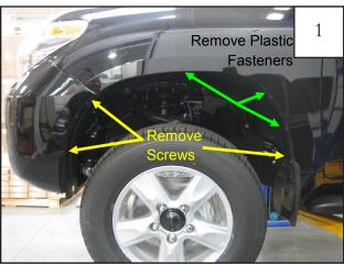
Using a socket with a T30 Torx bit, remove three factory screws. Use a trim tool or flat head screwdriver to remove three factory plastic fasteners located in rear of wheel well one located in the top center of wheel well. Discard.
