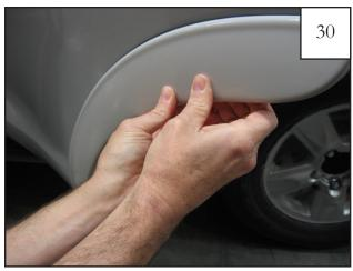
Brace fingers on inside of door and use thumbs to press firmly against part and repeat along full length of part at lower tape liner location. *Tape reaches maximum adhesive bond after 24 hours of contact.*
