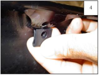
The splash shield needs to be pushed behind metal fastening point to access where the clip needs to be installed.
