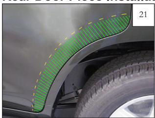
Using supplied alcohol wipe, clean area for door piece attachment.
