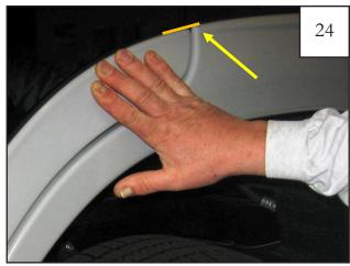
With door closed, line up the door piece rubber edge to line up with main rear rubber edge and mark the door with a grease pencil or piece of tape
