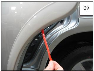
While holding Door Piece in place, pull lower tape liner tab.
