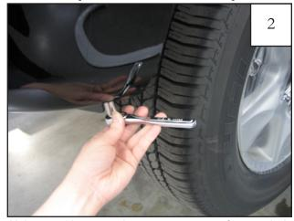
Using a 10mm socket, remove one factory bolt located at front underside of bumper. Discard.
