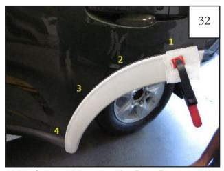
Using foam pad between the Door Piece and the ratcheting clamp, Attach clamp on upper part of Door Piece in position 1 and tighten. Leave clamp in place for 1 minute. Repeat clamping method for positions 2, 3 and 4. Leave clamp in place for 1 minute in each position.
