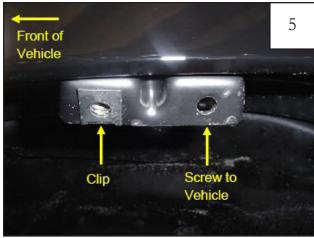
Install supplied plastic bracket using large Hex Screw into the plastic clip installed in step 10. The screw goes in rearward hole and the clip fastens over the forward hole.
