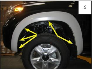
Reposition Front Flare on Fender. Hand start five supplied Hex Screws through flare and into hole locations shown (three in wheel well, one at front underside of bumper, and one through the "U" Clip installed on bracket in Step 11). Do not tighten.
