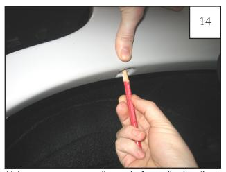
Using a grease pencil, mark four clip locations on fender of flare, using holes in flare as a guide. Remove screws and remove flare from fender.
