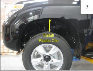
Install plastic clip onto factory sheet metal below the inner splash shield.
