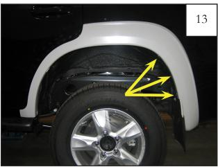
Position Rear Main Flare on fender, and hand start three supplied Hex Screws in rear of rear wheel well, starting with the top screw and working your way down.
